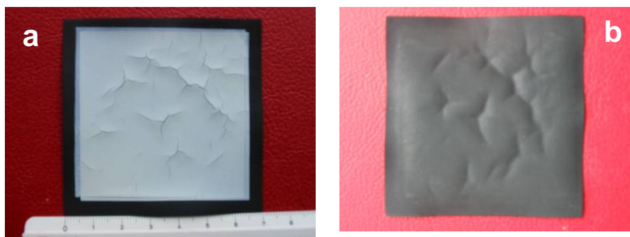
Figure 1. Photographs of the anode-electrolyte green bilayer taken five minutes after deposition. a) front, b) back.
