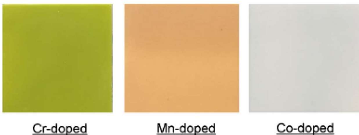
Fig. 10. Ceramic glazes prepared with Cr-doped (Cr14) Mn-doped (Mn5) and Co-doped (Co5) tialite pigments.
