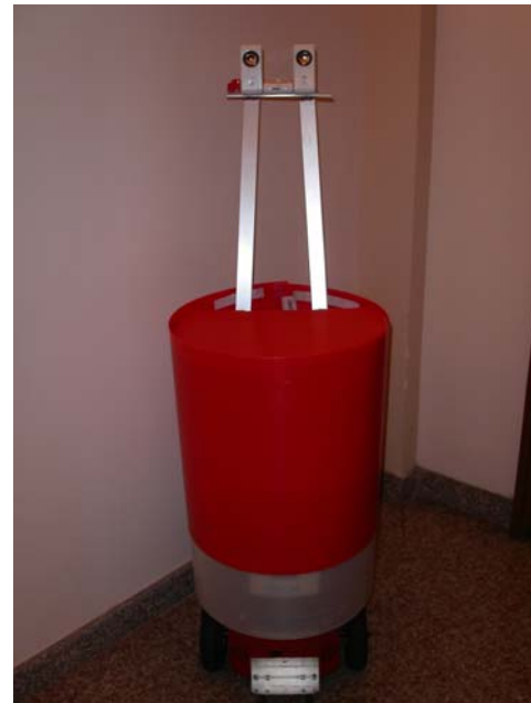
Figure 2b. Non anthropomorphic version of the robot
