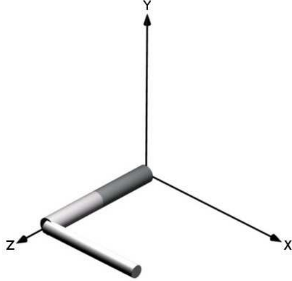
Figure 4: The starting position of the two simulated 3D/4DoF arms. The shown joint angles are taken as being at 0^\circ .
