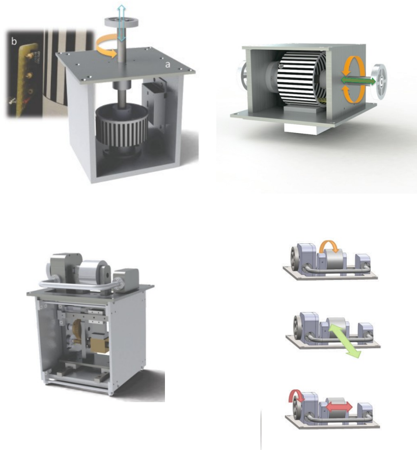
Fig. 3 (Up) On the left Circular Tap: (a) overall layout; (b) encoder electronics; On the right Fixed prism: the frontal wall has been removed allowing to see inner mechanism; (bottom) 3 Dof cylinder: overall layout (left); degrees of freedom (right): central wheel rotation; horizontal translation (middle); translation of the central wheel driven by lateral circular handle bottom
