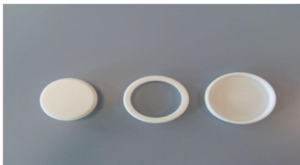
Figure-2. The passive sampling device Chemcatcher
