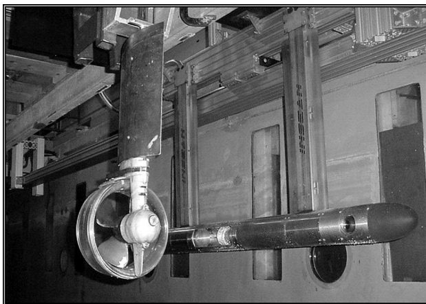
Fig. 1 DP thruster model and SPIV in the INSEAN large cavitation tunnel
