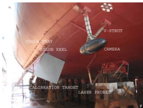
Figure 20 PIV setup on the Italian vessel, Nave Bettica , from Atsavapranee et al. (2008)
