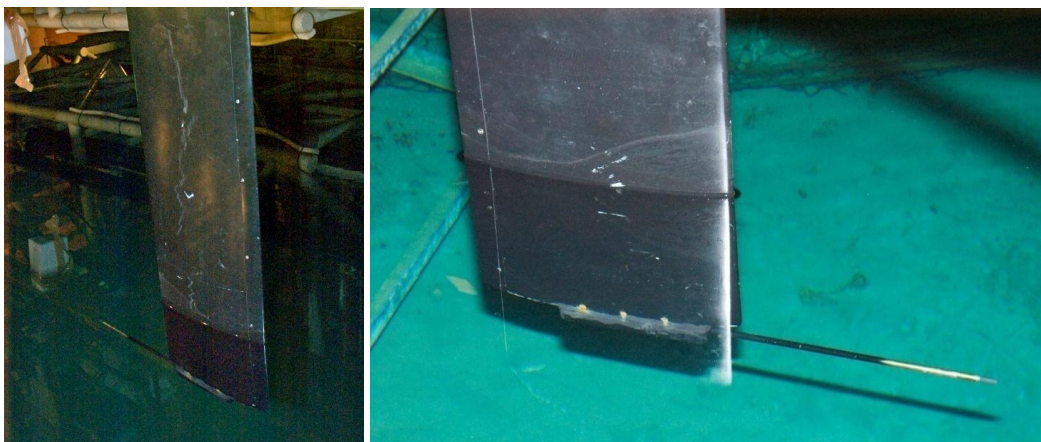
Figure 19. Detail of the strut supporting the in-flow sensor (hydrophone) and particular of the stem and the strut.
