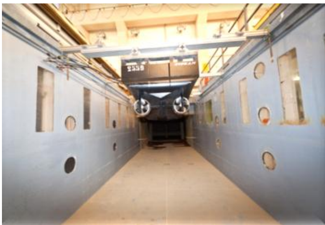
Figure 18: INSEAN large circulating water tunnel: test section
