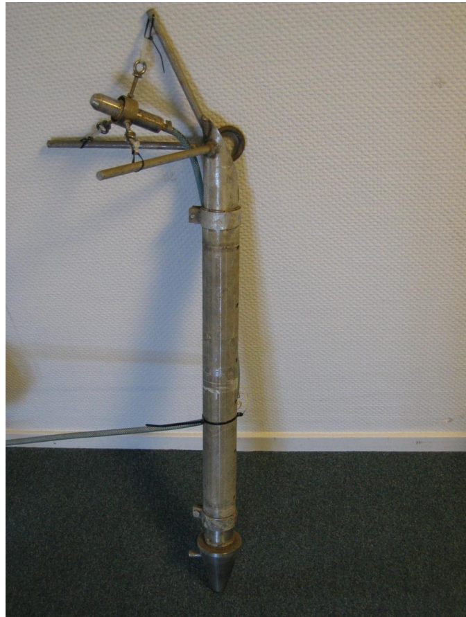
Figure 12: The beam hydrophone pole with the ZP84 hydrophone
