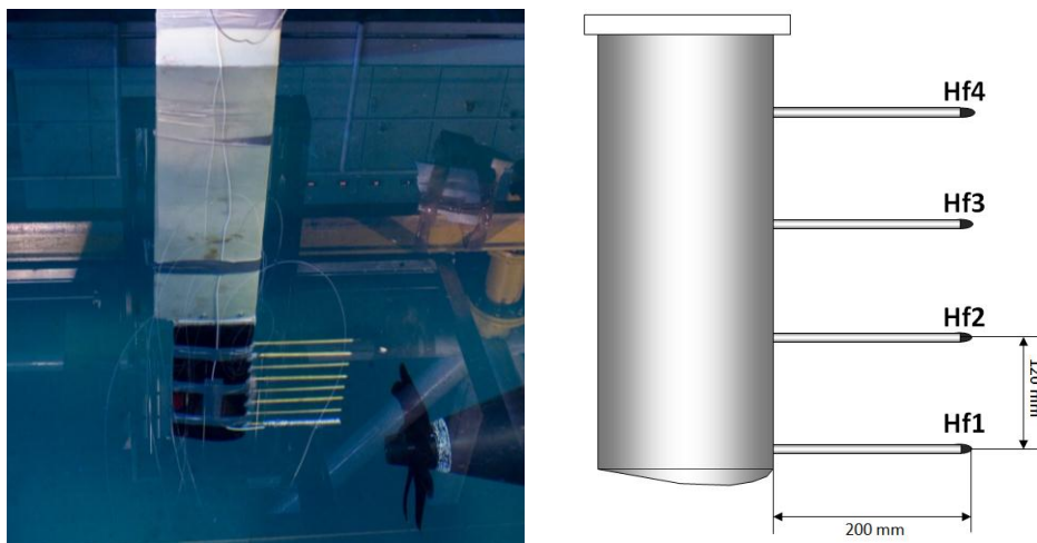
Figure 20. Hydrophone mounting on the rake device: picture (left) and geometrical representation (right) Hydrophones are also used to measure the flow noise levels on the model surface. In this regard, the transducers are fitted inside a cylindrical cavity, which is flush mounted with the outer shell of the model body. The cavity is designed to communicate with the flow through a 2-mm diameter hole, and is therefore filled with water (Figure 21).
