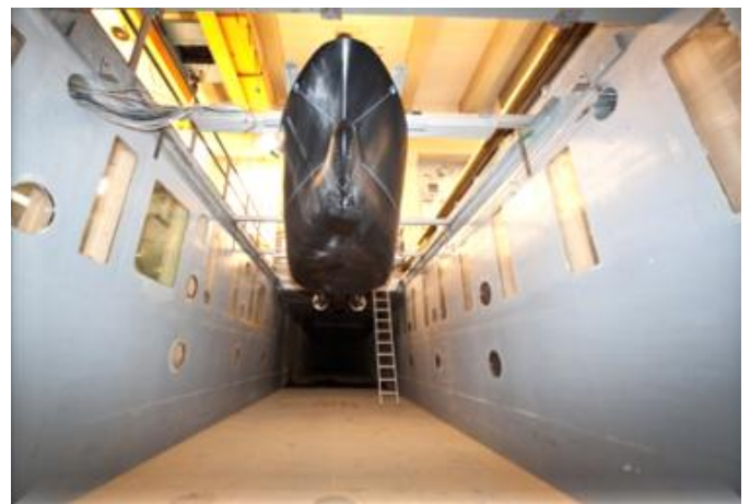
Figure 18: INSEAN large circulating water tunnel: test section
