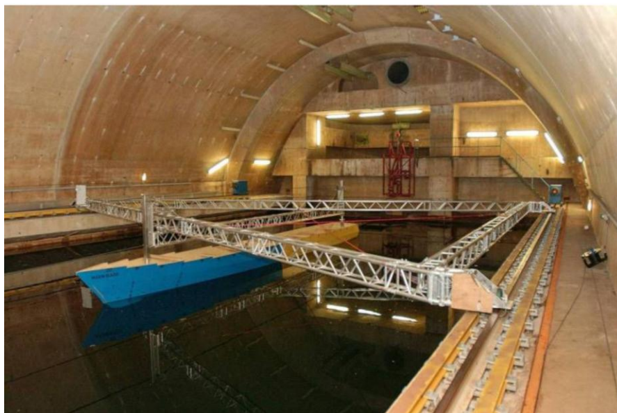
Figure 9. The silent towing system of MARIN.
