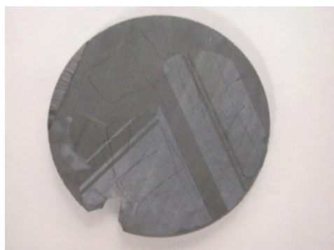
Radial section of ingot growth without Pt
