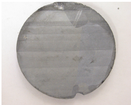
Fig.1. Wafer of the ingot grown by OBR with superheating conditions.
