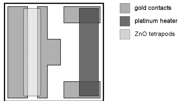
Figure 3. Schematic draw of the sensor contacts and heater geometry.
