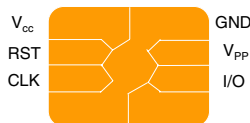
Fig. 1. Smart card chip and its connection points: supply voltage ( V_{CC} ), reset signal ( RST ), clock ( CLK ), ground connection ( GND ), input/output ( I/O ) and external voltage for programming ( V_{PP} , generally not used)
