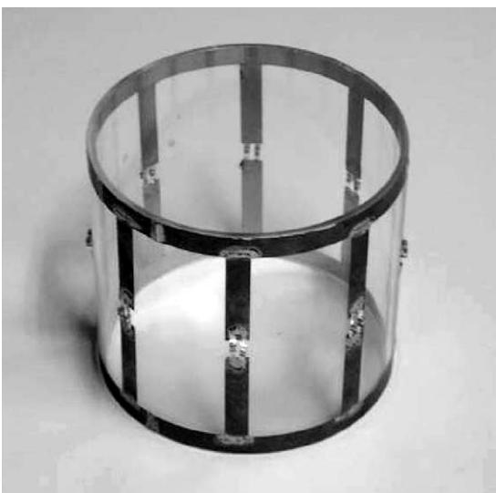
Fig. 11. Illustration of the built low-pass birdcage coil.
