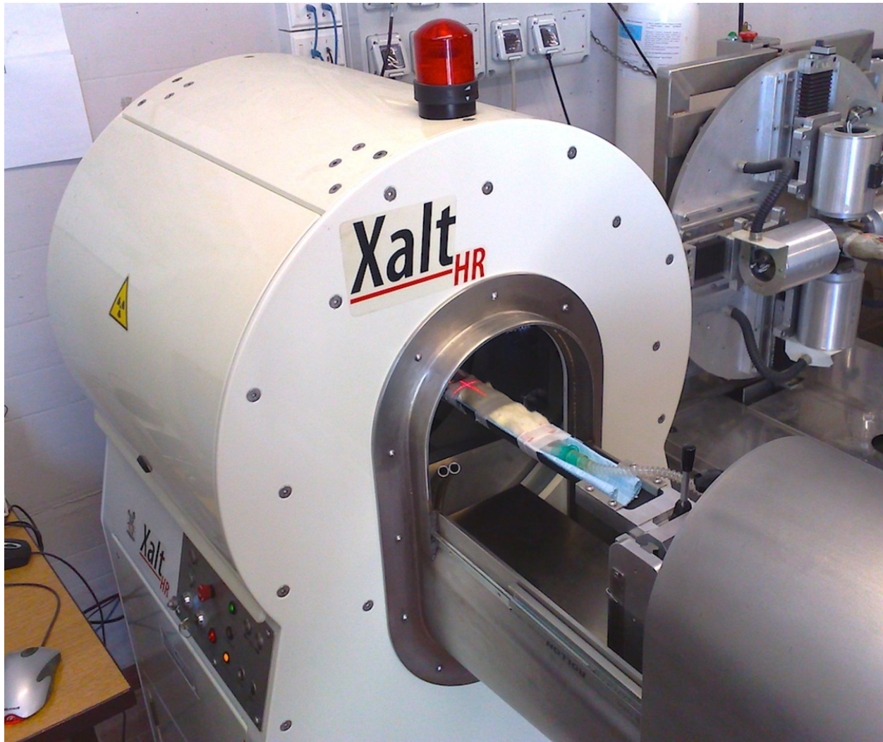
Fig. 2: The Xalt micro-CT scanner at the Molecular Imaging lab of IFC-CNR, during an animal study.
