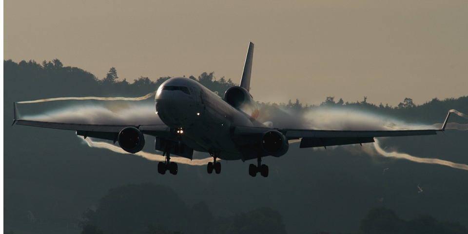
FIGURE 1.1: Contrails Created by an Extended Flap on a Transport Aircraft During Landing (Berens (2008))
