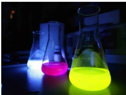
Figure 2-1 – Fluorescence: all the three liquids are excited with UV, but each emits at a different wavelength.
