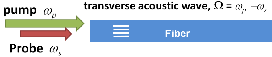
FIGURE 7.1: Forward stimulated Brillouin scattering in an optical fiber. The co-propagating optical beams are coupled to transverse vibrational modes in the optical fiber. The picture shows the signal beam on the Stokes side.
