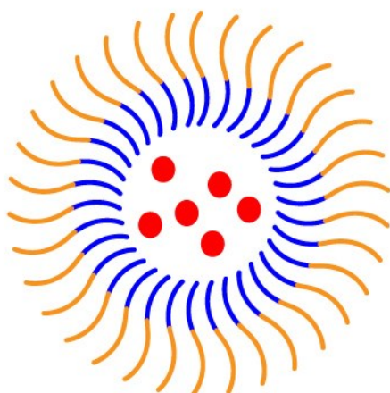
Figure 3: Diblock micelles with thermosensitive coronas. (A) At temperatures below the transition temperature of the thermosensitive polymer (orange; pNIPAAm), the hydrophilic
