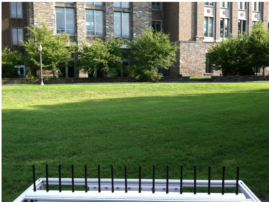
FIGURE 7.7: Setup of calibration experiment to obtain clutter training data
