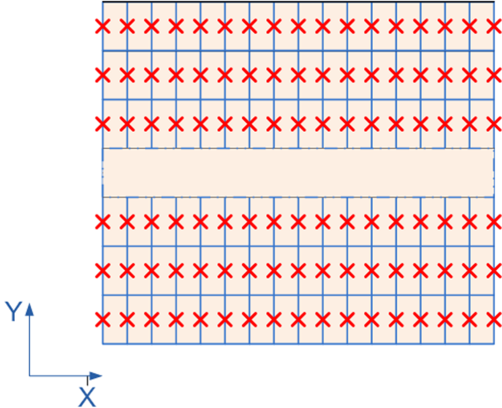
FIGURE 3.19: The 15 \times 20 rectangular SQIF array with a SQUID dimension of 10 \mu\text{m} \times 20 \mu\text{m}
