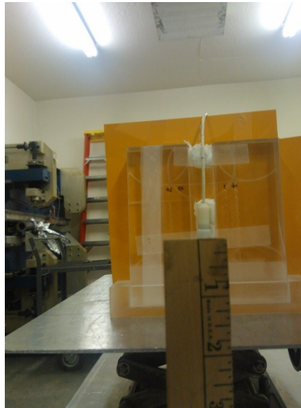
Figure 2.11: TLDs, film and ionization chamber with Plexiglas frame
