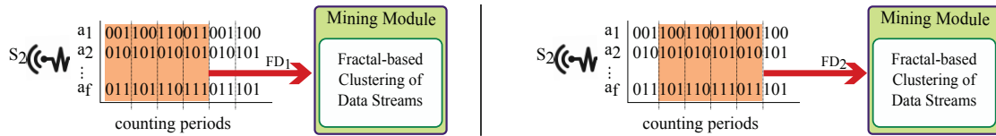
Figure 4. Sliding Window of a sensor, counting periods t = 4 , events e = 3 .
