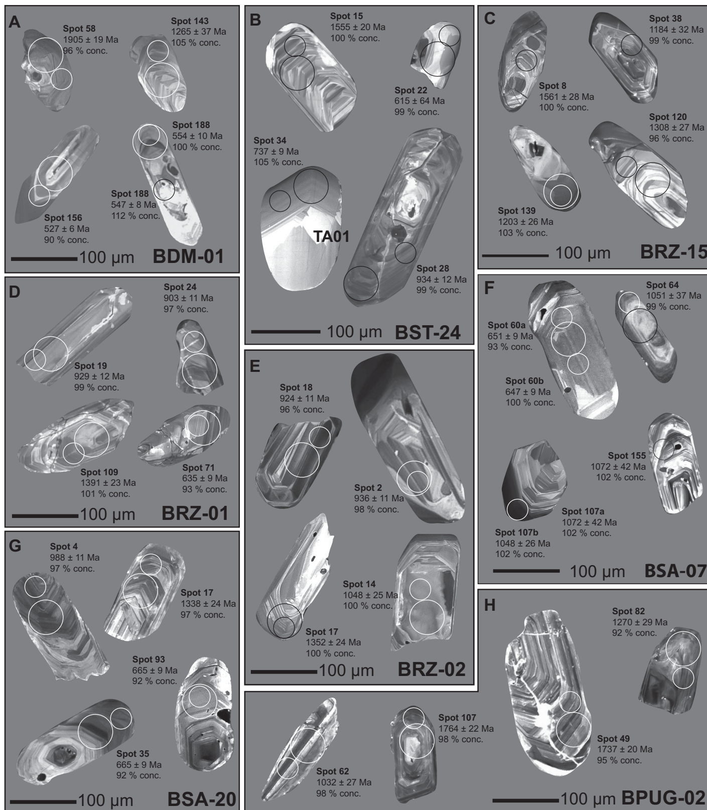
Figure 4. Cathodoluminescence images of representative zircon grains from sample (A) BDM-01; (B) BST-24; (C) BRZ-15; (D) BRZ-01; (E) BRZ-02; (F) BSA-07; (G) BSA-20; and (H) BPUG-02. Displayed spot ages younger than 1000 Ma and older than 1000 Ma are ^{206}\text{Pb}/^{238}\text{U} and ^{207}\text{Pb}/^{206}\text{Pb} ages, respectively. Small circles (30 \mu\text{m} ) and large circles (50 \mu\text{m} ) represent the locations of U-Pb and Lu-Hf analyses, respectively.
