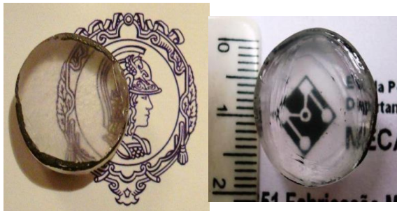
Figure 3. Transparent samples obtained from the sintering of crystalline powder (left) and amorphous powder (right).
