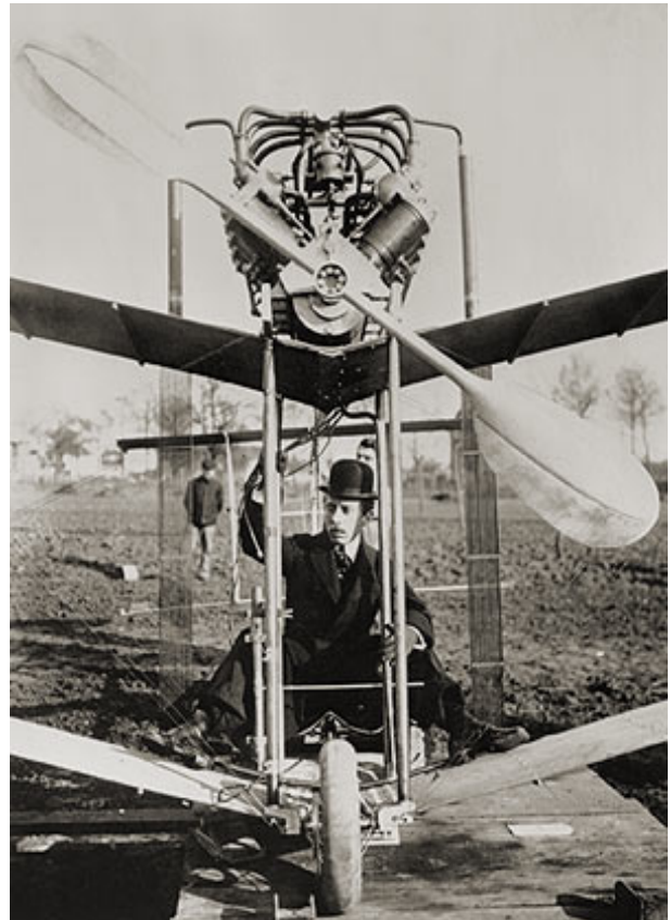
Fig. 4 Santos Dumont design #15 the undercarriage in wrong position did not allow rotation for take-off [10].
