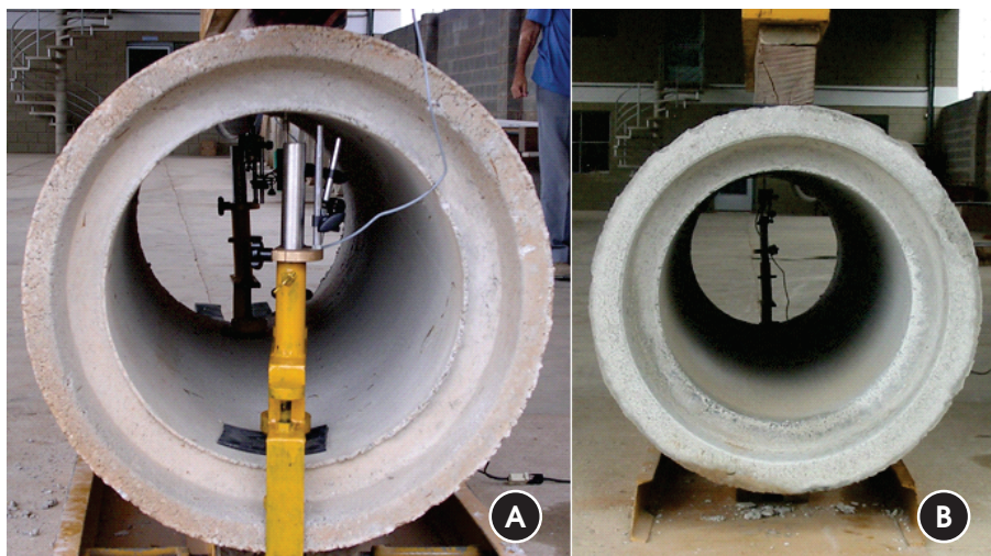
Figure 2 – Configurations adopted for the measurement of displacements (A) at both extremities in the 1 st Series and (B) at the spigot for the 2 nd Series
