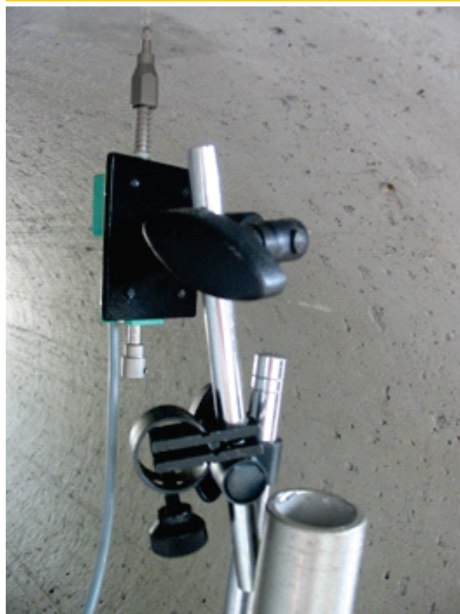
Figure 3 – LVDT positioned at the upper part of the inner surface of the pipe
