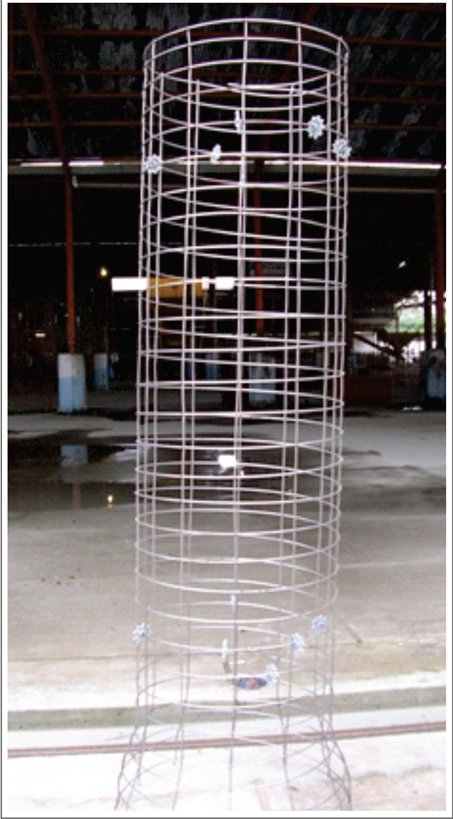
Figure 4 – Rebars set up used in SBRCP production that served as a parameter for comparative performance evaluation with FRCP
