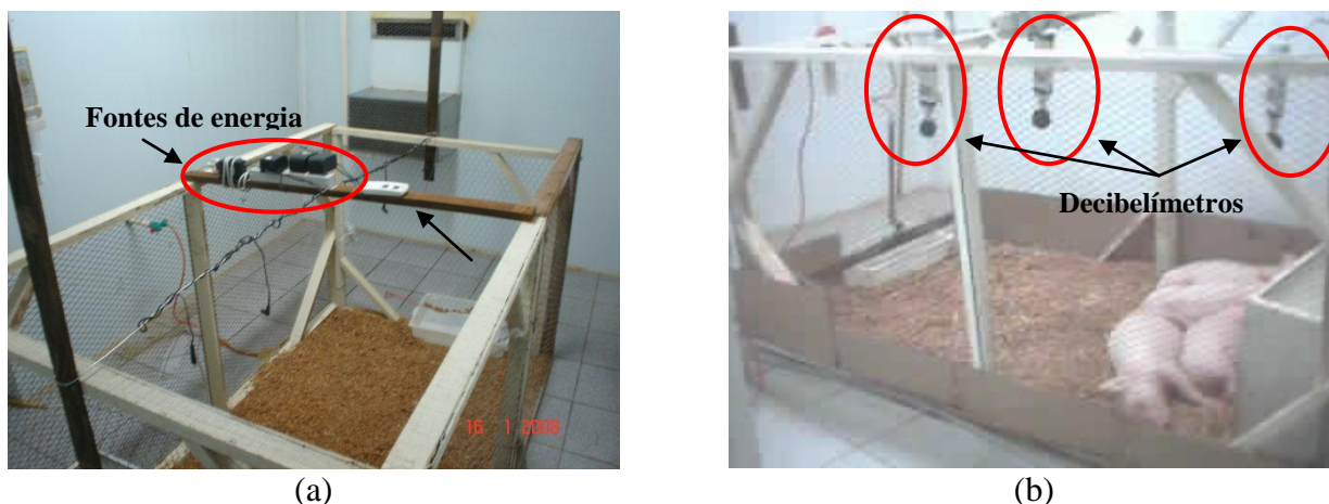
FIGURA 2. (a) Fontes para energizar os decibelímetros. (b) Locação dos decibelímetros no interior da câmara climática. (a) Power to supply the sound meter levels. (b) Location of the sound level meters inside the environmental control room.
