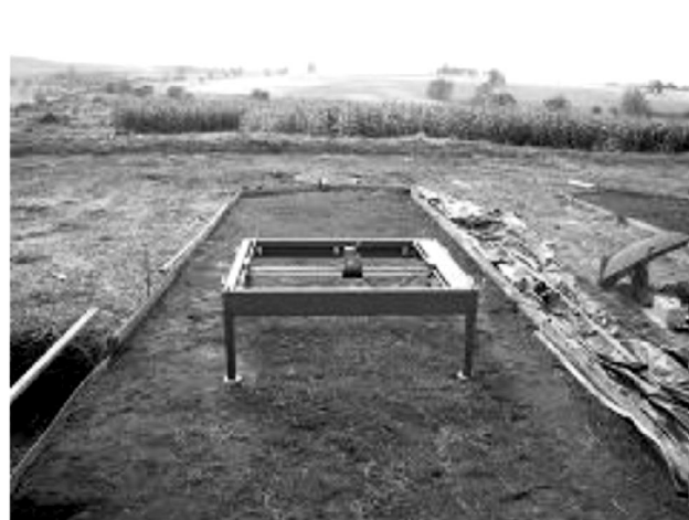
Figure 1. Laser profile scanner installed on one of the experimental plots.
