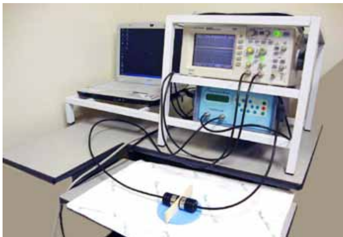
Figure 3. Measurement of ultrasound velocity via the transverse direct contact technique.
