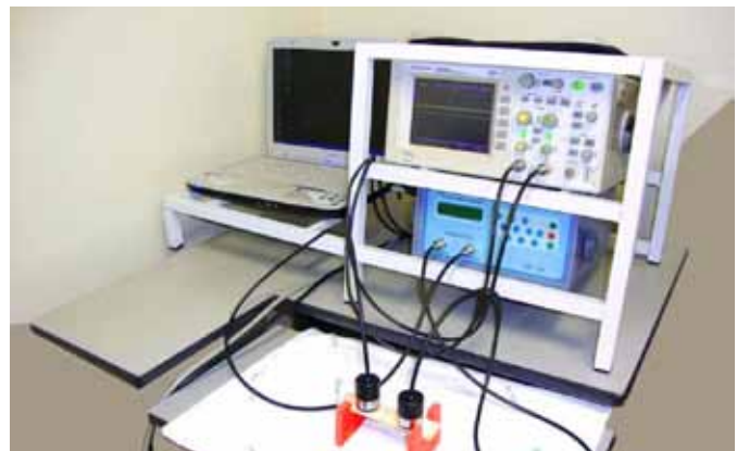
Figure 2. Measurement of ultrasound velocity via the axial direct contact technique.
