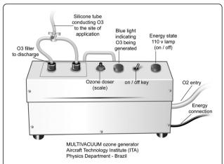
Figure 2 Schematic representation of a medicinal  $O_3$  generator equipped with an oxygen flow controller with 0.01 min precision, in which a controlled oxygen flow passes through a glass cylinder and is exposed to an electric discharge by a dielectric barrier with controlled potency and voltage.
