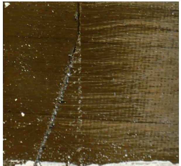
Fig. 10. Failure of off-axis [15] 10 under compression loads.
