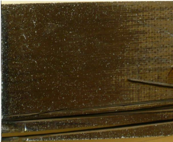
Fig. 8. Failure of off-axis [5] 10 under tension loads.
