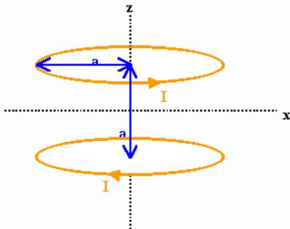
Figura 1 - Ref. [9]: Par de bobinas no arranjo anti-Helmholtz.
