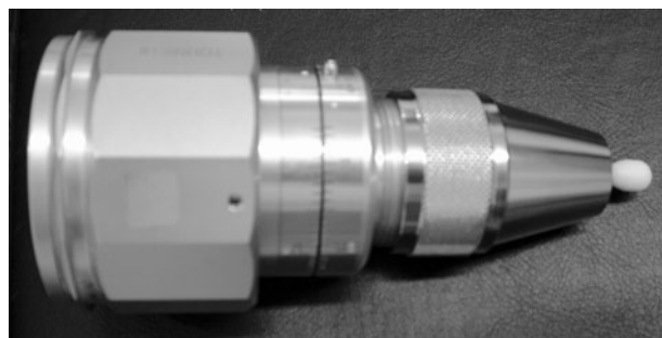
Figure 2. Implant-abutment clamped in the Tohnichi torque meter with the Torqtite screw. The abutment screw is tightened with the head of the Torque Controller.
