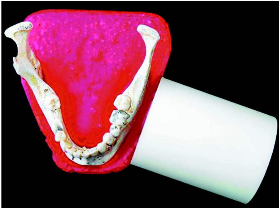
FIGURE 1- Mandible on acrylic base for standardization of x-ray incidence angle and position of the optical plate
