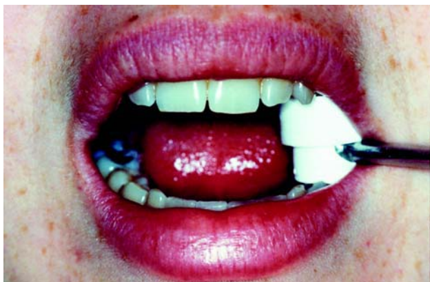
FIGURE 4- Bite force sensor at measurement position. The maximum isometric bite force was quantified at points where the subject felt safer to develop the maximum strength
