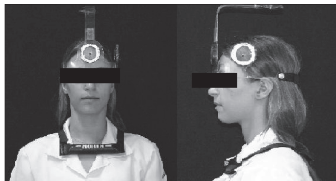
Figura 1. Cervical Range of Motion (CROM, Performance Attainment Associates, T Paul, MN USA) no plano frontal (A) e no plano sagital (B).
