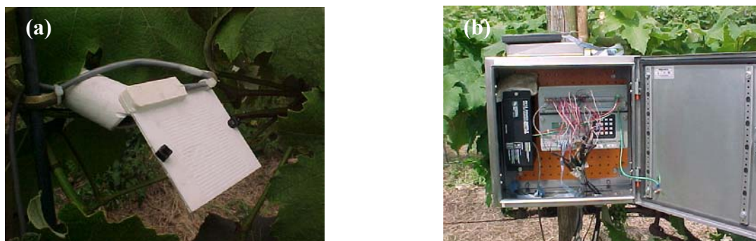
FIGURE 2. Detail of a flat plate wetness sensor (a) and the datalogger (b) inside the vineyard, in Jundiaí, SP, Brazil.
