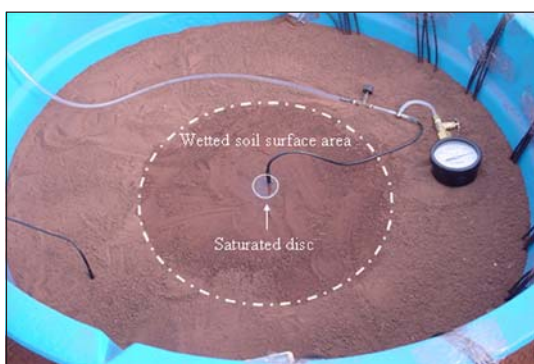
Figure 4 - Saturated disc and wetted soil surface area.
