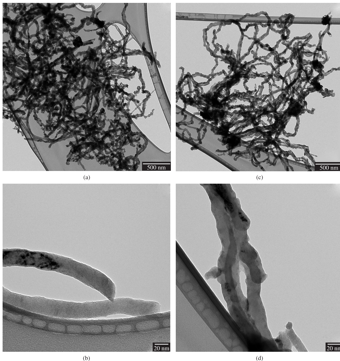
Figure 4. TEM images of catalyzed materials using SBR using: 17% of O_2 (a and b) and 19% of O_2 (c and d).
