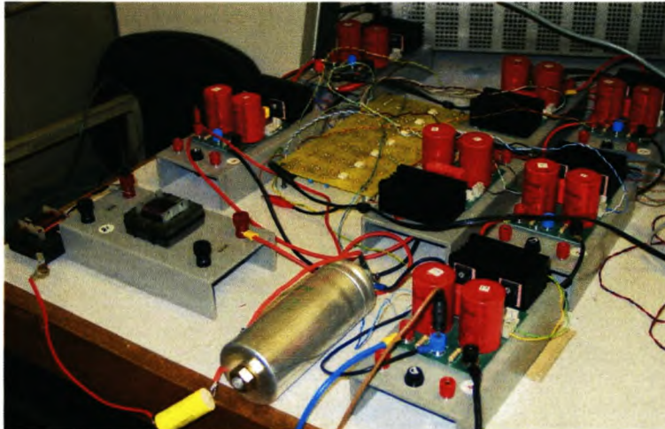
Figure 8.5: A picture of an eight-level FCMLI experimental prototype.
