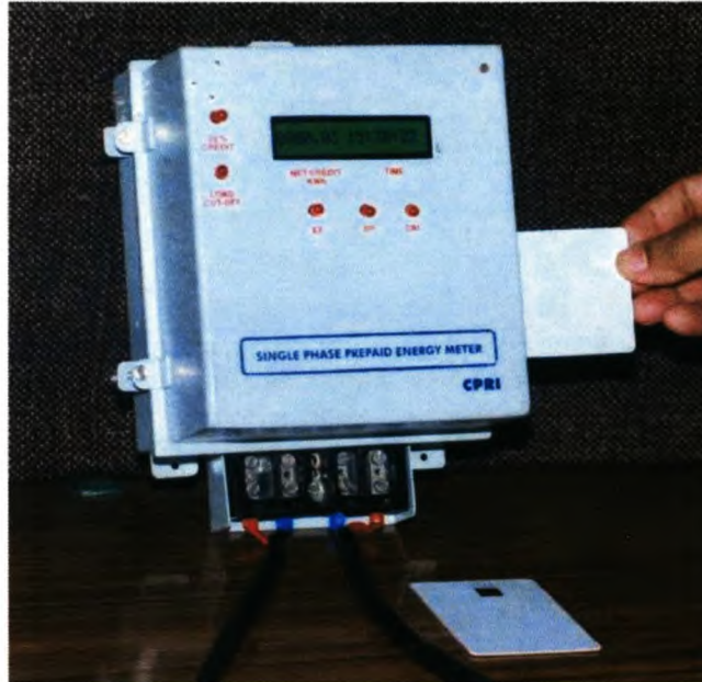
Figure 1.3: A single phase prepaid metering unit.
