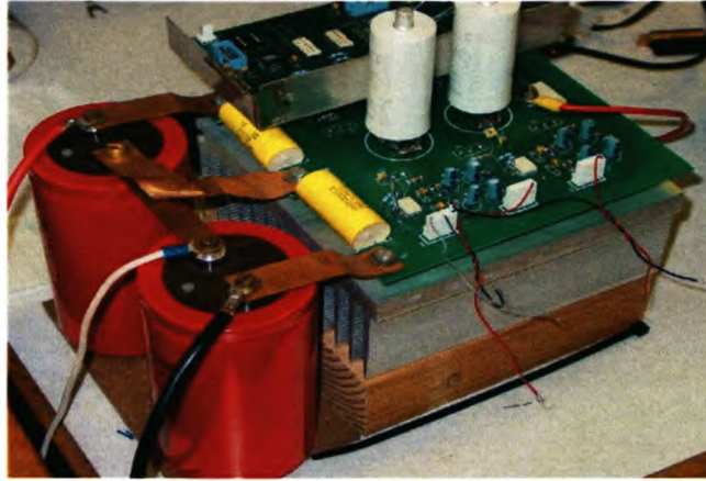
Figure 8.14: A picture of the experimental prototype of a four-level FCMLI.
