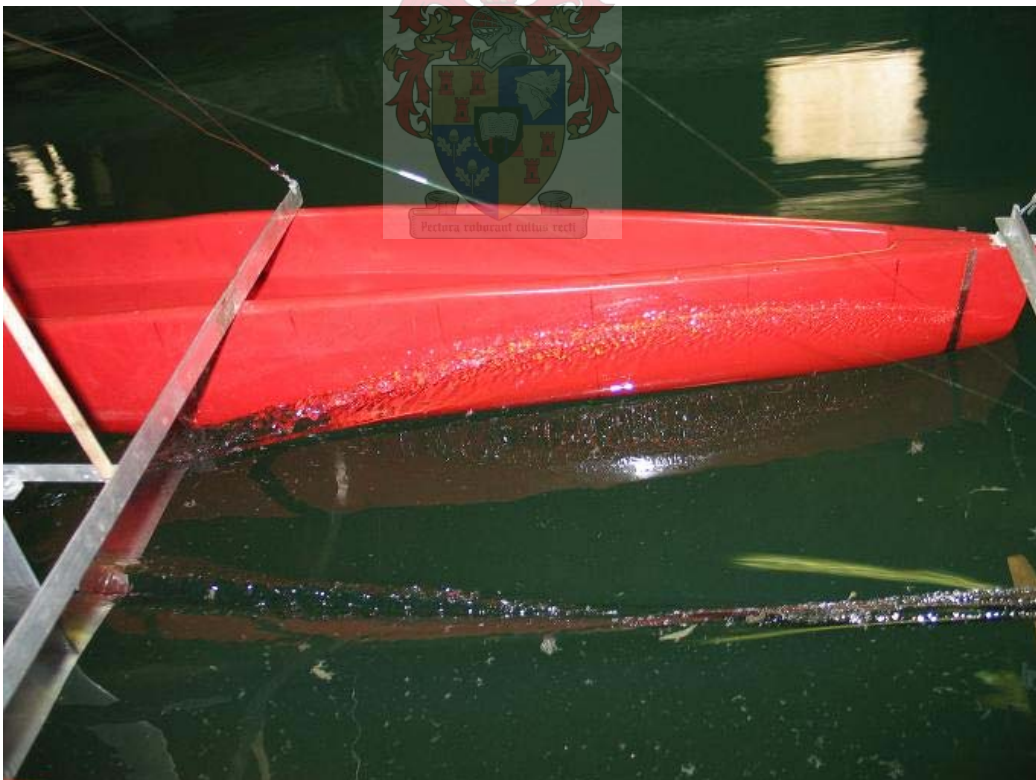
Figure E.8 d) Side view of nose down running condition Model Speed – 3.5 m/s ( \approx 19 knots full scale) Close to pitchpole at similar speed to without lifting foils
