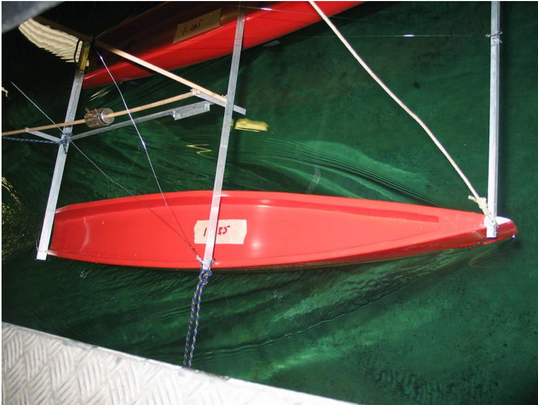
Figure E.4c) Wave pattern on leeward hull with 70^\circ heel angle Windward hull just emerged
