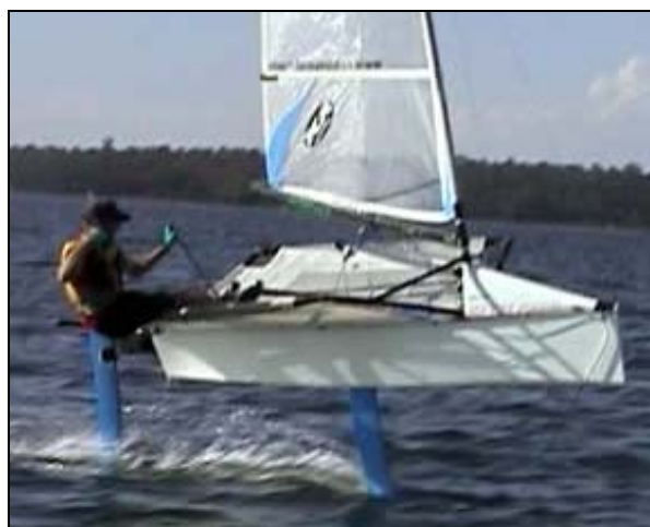
Figure 1.11 – Pictures of Veal's Moth [Vea05] Aircraft configuration, fully submerged foils and trim and ride height control
