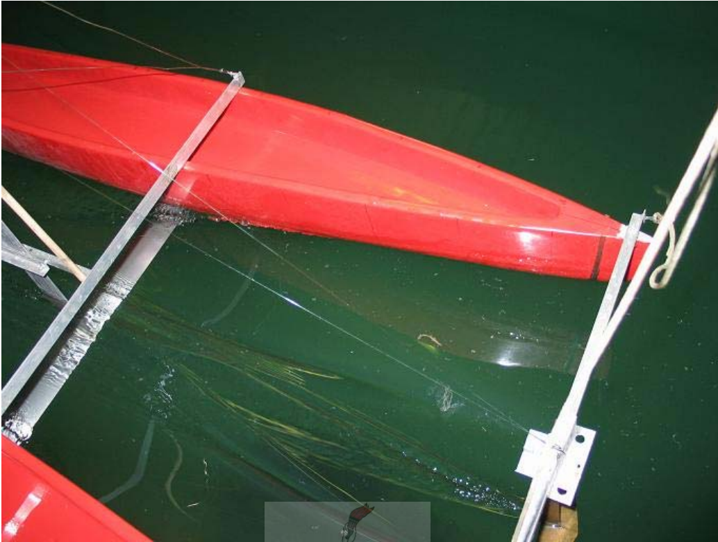
Figure E.8 a) Side of 'nose-up' running condition Model Speed – 2.0 m/s ( \approx 11 knots full scale)
