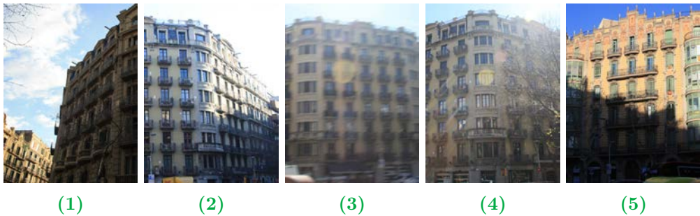
Figure 5.1: Illustrating different artifact sources, which are related to the capturing process. From left to right: (1) High-dynamic range scene with both shadowed and bright areas. (2) Completely saturated regions appear on the side of a facade. (3) Motion blur on an image taken with a handheld camera. (4) Lens flares. (5) Strong shadows cast by the Sun.
