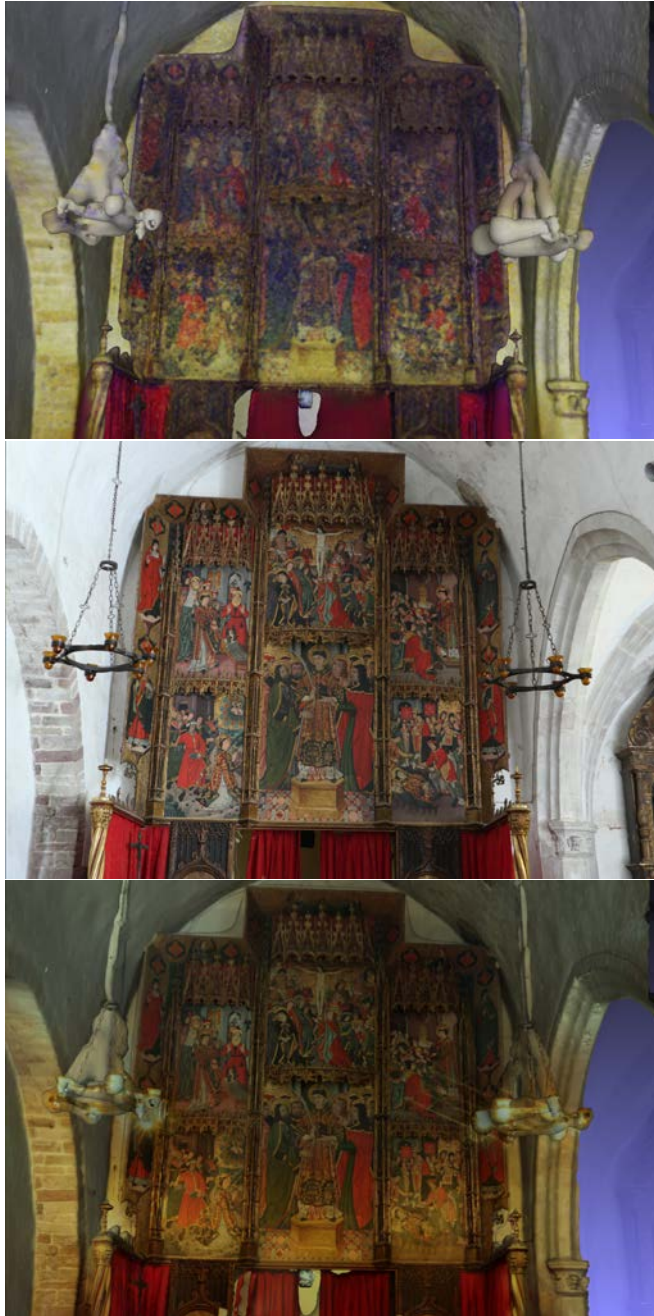
Figure 5.31: Altarpiece from “La Doma” church at La Garriga (Barcelona). From top to bottom: (1) Original mesh color (extracted from the panoramas captured at scan time), (2) sample photograph registered to the geometry and (3) resulting color from projecting the different images onto the mesh.
