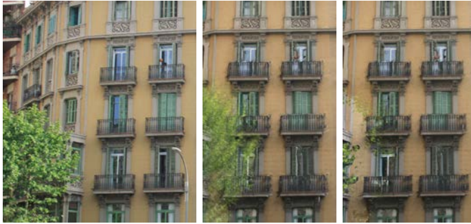
Figure 5.4: Despite depth tests, colors from occluding objects such as tree leaves often contribute to facade textures. The contribution is specially noticeable in those parts captured from a few unoccluded views. From left to right: (1) Photo a building. (2) Reconstruction (Colmap + image reprojection); notice tree color on the facade. (3) Removing reconstructed trees before reprojection increases color pollution because of the lack of depth test rejections.
