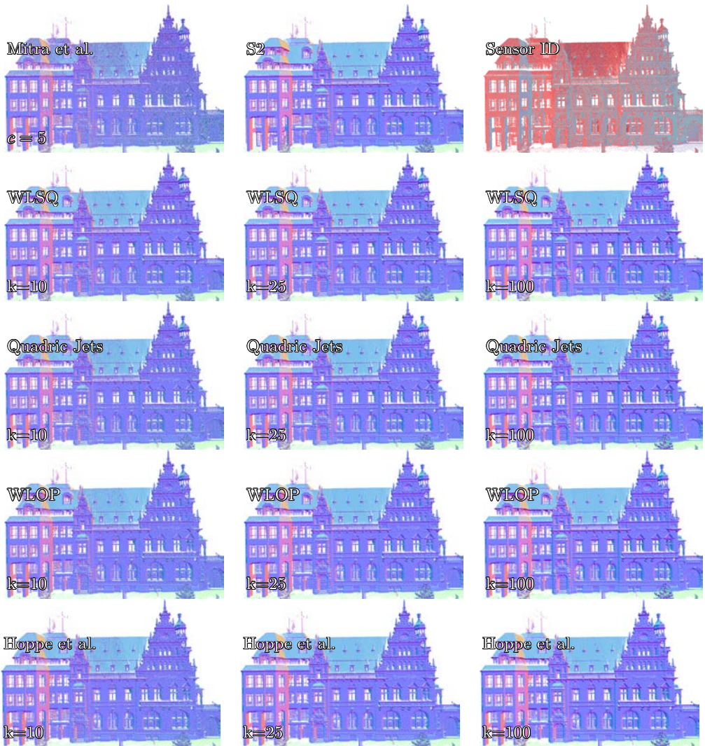
Figure 4.25: Evaluation of our results on real data. Images show estimated normals. From top to bottom: different algorithm including (1) Mitra et al. [MN03] and our proposed (S2) (Covariance Correction) (2) Our proposed (WLSQ) estimation. (3) Quadric Jets [CP05] (4) WLOP [HLZ+09] (5) Hoppe et al. [HDD+92]. This LiDAR point cloud recorded by Dorit Borrmann and Jan Elseberg from Jacobs University Bremen gGmbH, Germany [12]. It was captured using a Riegl VZ400 Scanner, with an accuracy of 0.5mm at 100m.
