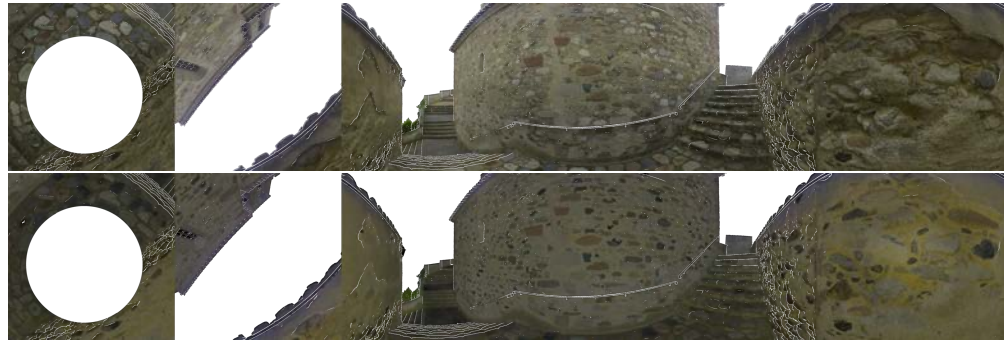
Figure 4.39: Showing the effects of our color enhancement strategy on a cloud captured with a Leica RTC 360. Because reflected IR intensity is less sensitive to illumination conditions our strategy lighting effects (shadows, highlights) making the depicted stone wall appear flat.
