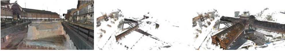
Figure 6.3: From left to right: (1) A single panorama rendered from its center point (2) The same panorama rendered from a distant point (3) Adding additional panoramas to improve coverage and allow for free camera navigation. The original sensor locations are shown as color spheres.
