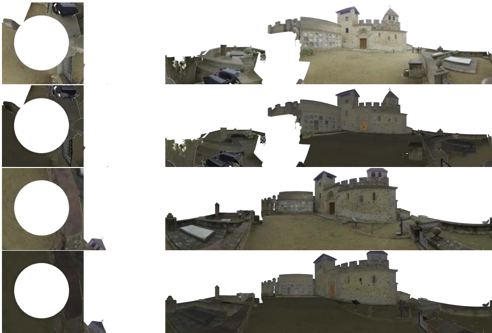
Figure 4.40: Showing the effects of our color enhancement strategy for different clouds of the same scene captured with a Leica RTC 360. Rows (1) and (3) show original color and rows (2) and (4) show the corresponding enhanced color. This scanner usually produces fewer color artifacts since it provides HDR images. Namely, it combines different image captures with different exposure settings for the same fragment of the scene. This scene was captured on a cloudy day. This is a usually good setting for outdoor scenes since diffuse illumination avoids the appearance of hard shadows and highlights. Nevertheless, we can see how one scan (1) appears clearly brighter than the other (3). Our strategy can make their color more consistent.
