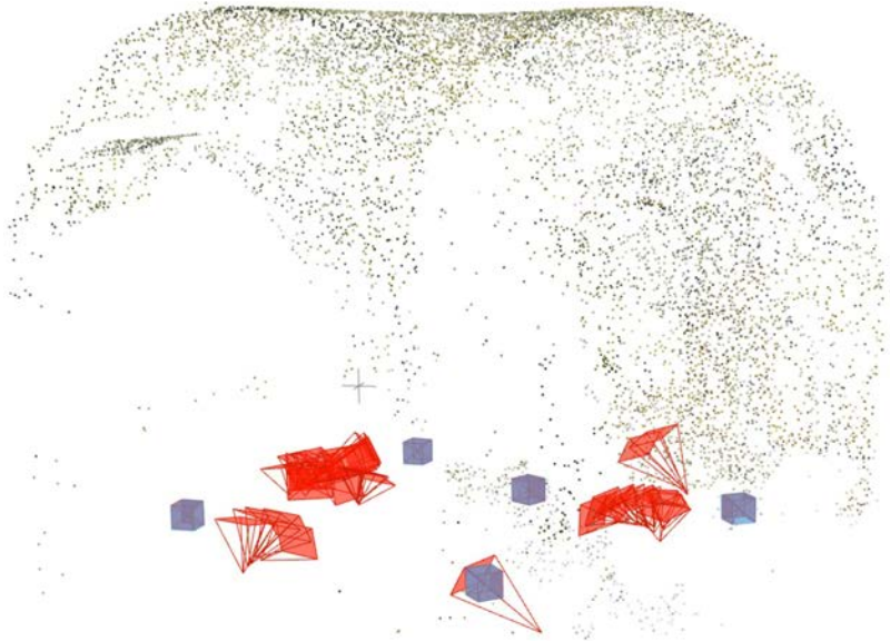
Figure 5.29: Sparse point cloud, cameras corresponding to cubemap images (in blue) and estimated camera poses for user-provided images (in red).
