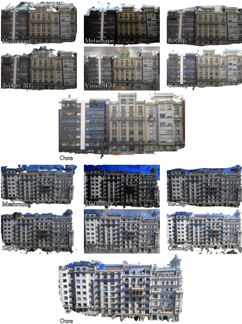
Figure 5.26: Comparison between different photogrammetry software, such as Alicevision Meshroom [MMM12; JP11], Agisoft Metashape Pro 1.5.5 [1], Autodesk ReCap Photo 2020 [2], 3DFlow Zephyr [STM+19; TGF+15], VisualSFM [WAC+11; Wu13]+CMVS+Meshlab [CCC+08], Colmap [SF16; SZP+16], and our pipeline.
