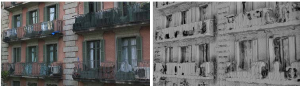
Figure 5.5: High-frequency facade elements such as balcony rails often cause sharp depth discontinuities between the rails and the wall. From left to right: (1) Photogrammetric reconstruction (Colmap) with reconstructed colors. (2) Same reconstruction using uniform color. An ambient occlusion term has been added to emphasize depth discontinuities.
