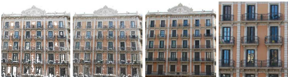
Figure 5.22: Impact of depth map repairing. From left to right: (1) Point cloud from original depth maps. (2) Point cloud from repaired depth maps. (3) Reconstructed mesh. (4) Close-up view.
