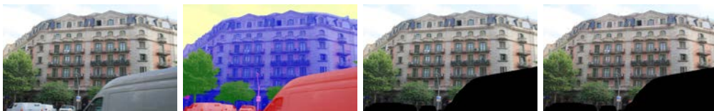
Figure 5.19: Moving objects such as vehicles lead to inconsistent feature matches between image pairs. We identify pixels belonging to vehicles and pedestrians and minimize their influence on image features.
