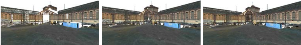
Figure 6.4: Combining multiple panoramas to improve coverage. From left to right: (1) a single panorama (2) 2 panoramas (3) 5 panoramas.
