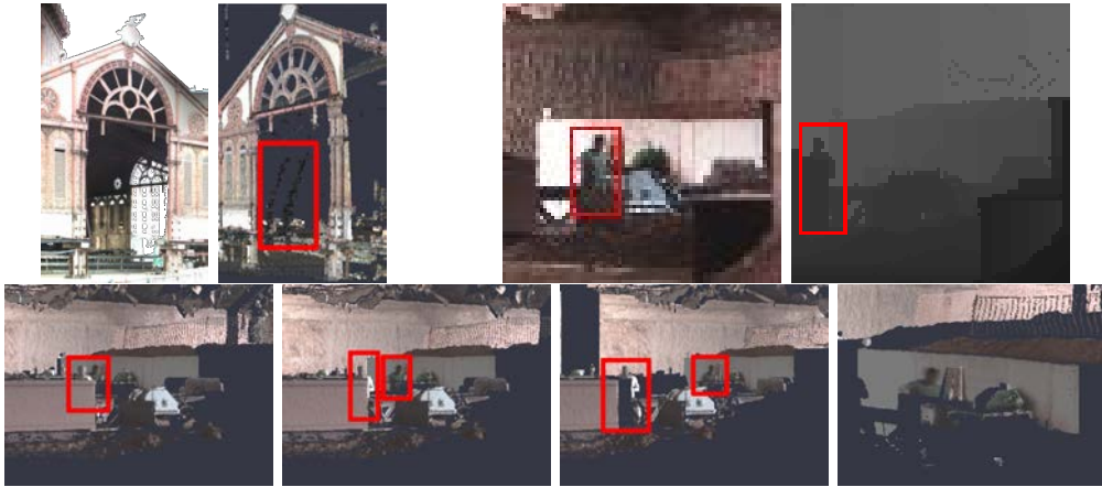
Figure 4.36: First row, from left to right: (1,2) Respectively, color image and render of the same cloud. In the render we can see a floating object that is not present in the color image. (3,4) Color and depth mismatch due to motion. Second row, from left to right: (5,6,7) Cloud renders from slightly different view points. The mismatch between geometry and color can be clearly seen. (8) Not a Banksy painting. This is a “false positives” artifact, a person captured only in the color images that has been pasted onto a wall.
