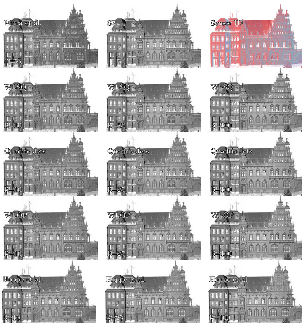
Figure 4.26: Evaluation of our results on real data. Images show shading using estimated normals. From top to bottom: different algorithm including (1) Mitra et al. [MN03] and our proposed (S2) (Covariance Correction) (2) Our proposed (WLSQ) estimation. (3) Quadric Jets [CP05] (4) WLOP [HLZ+09] (5) Hoppe et al. [HDD+92]. This LiDAR point cloud recorded by Dorit Borrmann and Jan Elseberg from Jacobs University Bremen gGmbH, Germany [12]. It was captured using a Riegl VZ400 Scanner, with an accuracy of 0.5mm at 100m.
