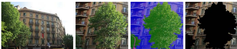
Figure 5.18: These two images capture usable scene content from two slightly different viewpoints. Since the tree occupies most of the overlap region, masking it before feature extraction would result in no feature matches between them.
