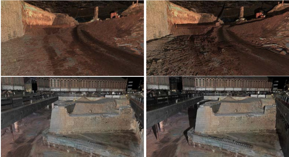
Figure 6.1: Panoramas rendered without (left) and with (right) shadow mapping (mesh-based rendering). For single panoramas, shadows are only accurate for light sources nearby the sensor location.
