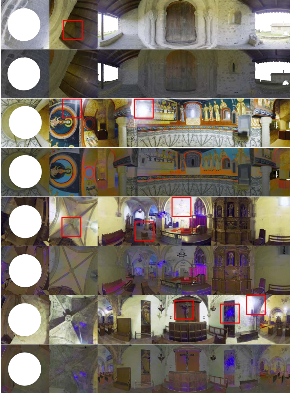
Figure 4.41: Showing the color artifacts produced by the Leica RTC 360. Zooms are shown and discussed in Figure 4.42.
