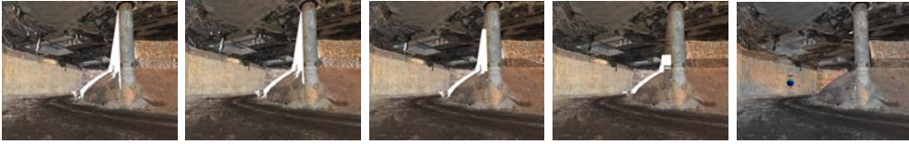
Figure 6.5: Panoramas rendered from an offset from the sensor location, with varying depth thresholds \varepsilon_d . From left to right: (1) \varepsilon_d = 50 cm (2) \varepsilon_d = 1 m (3) \varepsilon_d = 4 m (4) \varepsilon_d = 16 m (5) \varepsilon_d = 50 cm (two panoramas).
