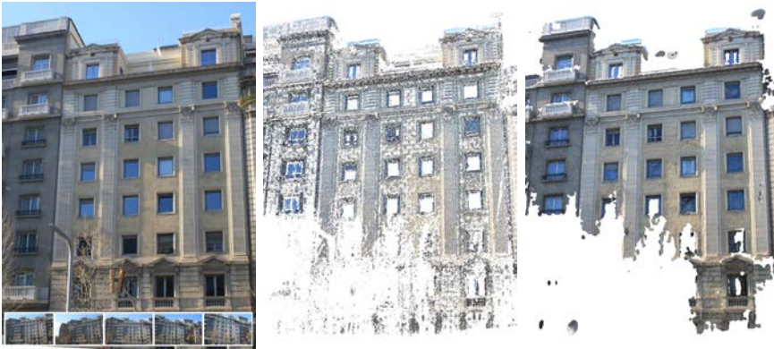
Figure 5.2: Example of poor reconstruction of low-texture parts. The reconstructed dense point cloud (Colmap) has important missing parts which are not recovered through meshing.
