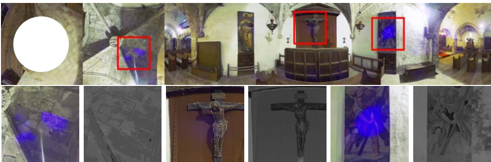
Figure 4.35: Showing the color artifacts produced by the Leica RTC 360. Lens flares typically appear on images captured in scene with very bright sources. These are usually caused by the internal light refraction and scattering on imperfections of the lenses. In these images we can see several lens flares due to the scanner mosaicing strategy, namely composing several images into a single one.
