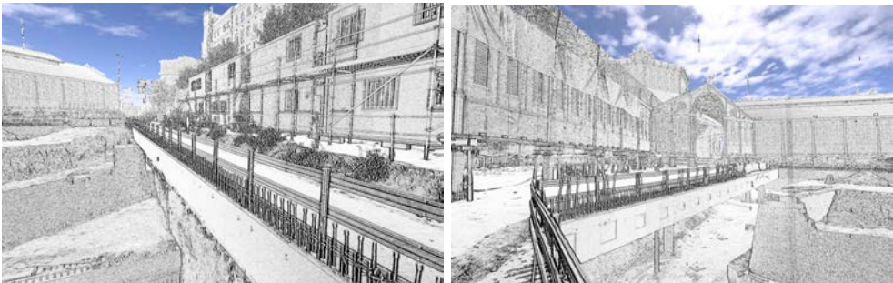
Figure 6.2: Panoramas rendered with an illustrative shader based on Screen-Space Ambient Occlusion with small radius. Robust normals are essential for getting good estimates of the ambient occlusion term.
