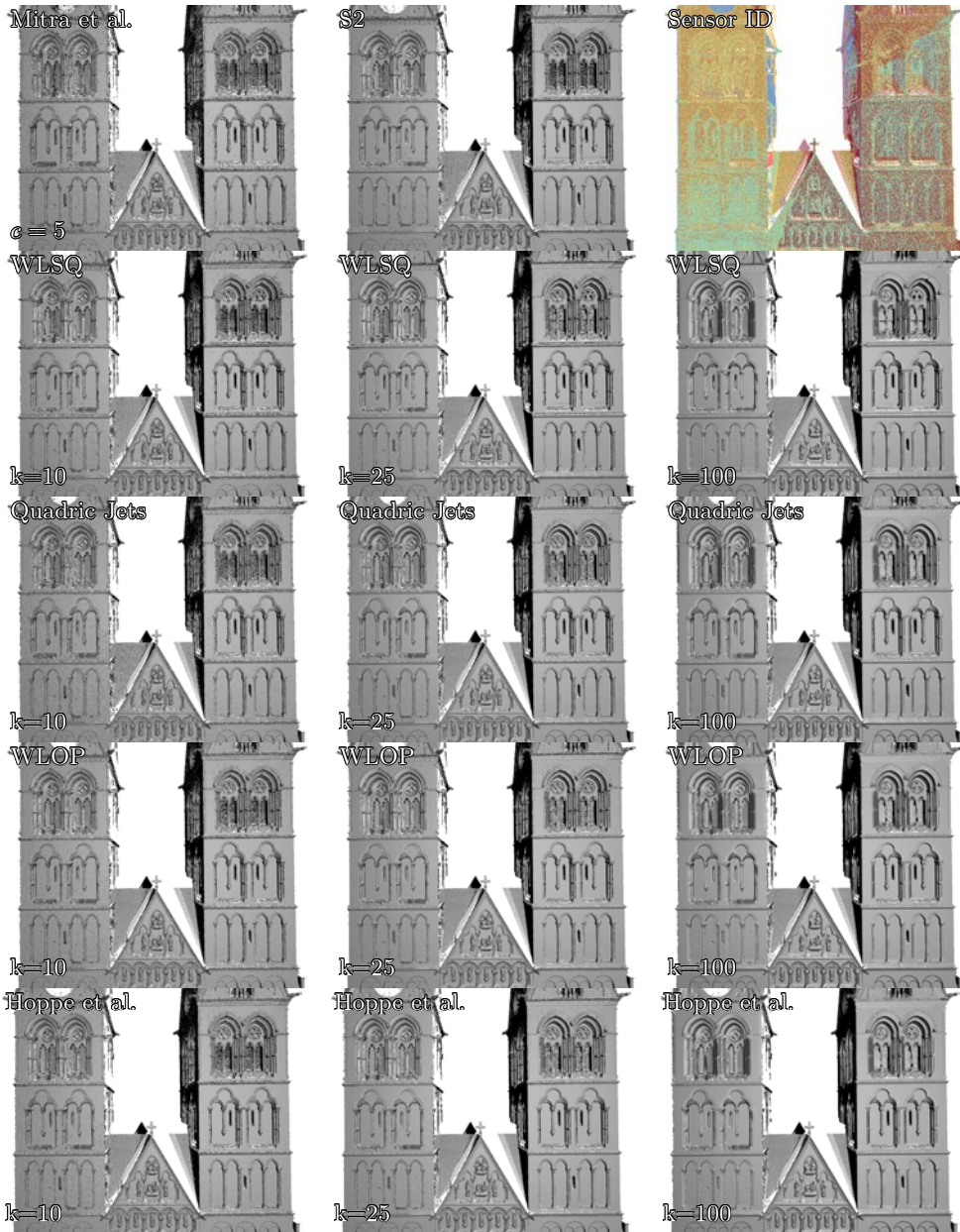
Figure 4.28: Evaluation of our results on real data. Images show shading using estimated normals. From top to bottom: different algorithm including (1) Mitra et al. [MN03] and our proposed (S2) (Covariance Correction) (2) Our proposed (WLSQ) estimation. (3) Quadric Jets [CP05] (4) WLOP [HLZ+09] (5) Hoppe et al. [HDD+92]. This LiDAR point cloud recorded by Dorit Borrmann and Jan Elseberg from Jacobs University Bremen gGmbH, Germany [12]. It was captured using a Riegl VZ400 Scanner, with an accuracy of 0.5mm at 100m.
