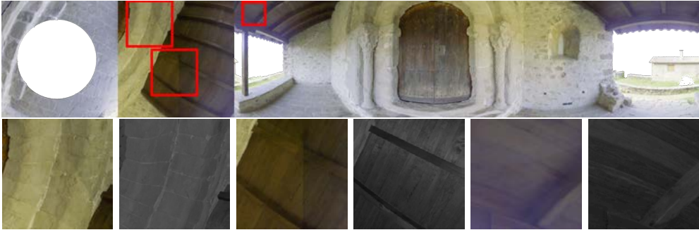
Figure 4.34: Showing the color artifacts produced by the Leica RTC 360. This system captures HDR images, which greatly improves color consistency. Nevertheless, some sharp color discontinuities can still be seen in these images.
