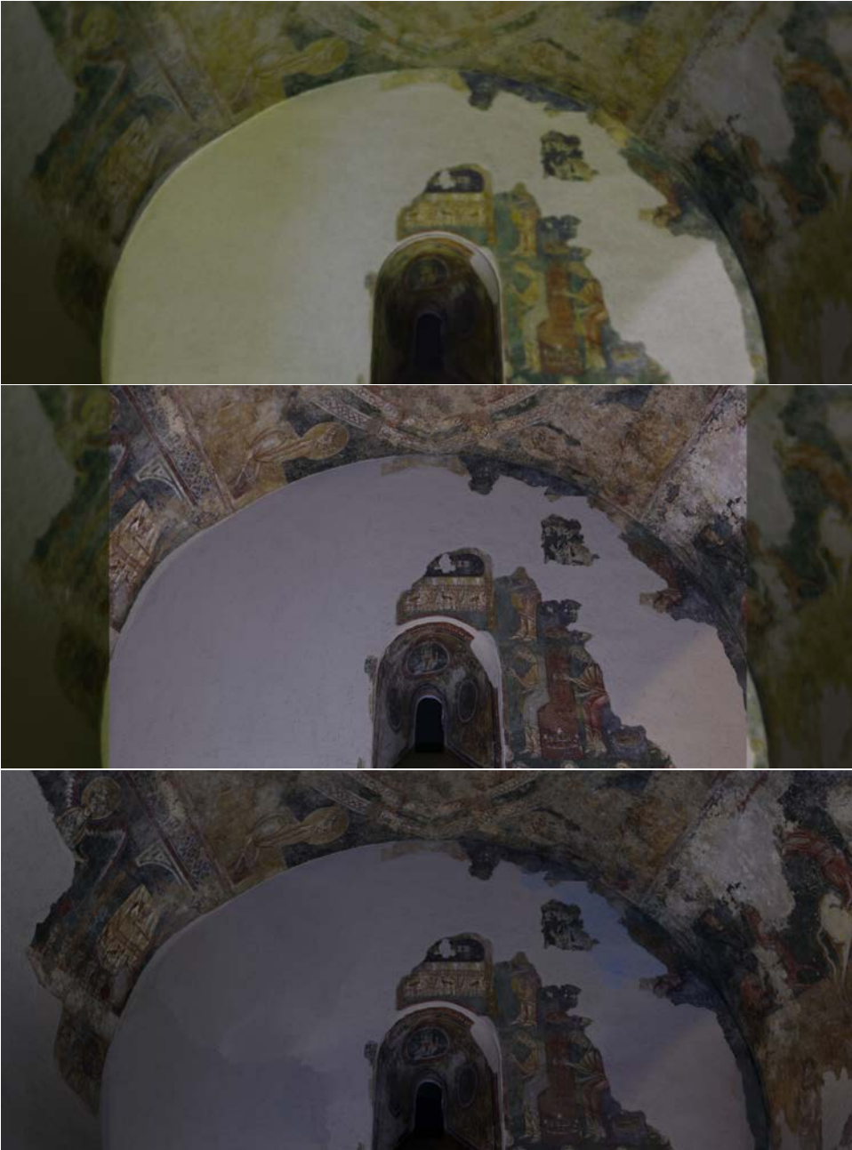
Figure 5.30: Small slice of the museum model (Museu Diocesà i Comarcal de Solsona). From top to bottom: (1) Original mesh color (extracted from the panoramas captured at scan time), (2) sample photograph registered to the geometry and (3) resulting color from projecting the different images onto the mesh.
