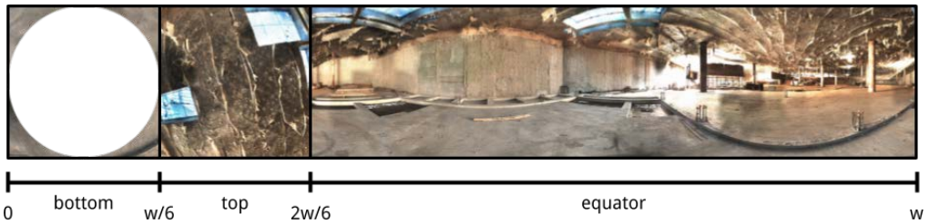
Figure 4.32: Stretch-invariant polar capped color map for a given scan.
