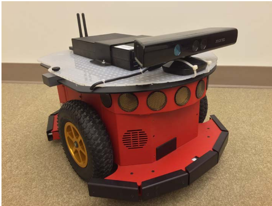
Figure 7. The Pioneer P3-DX with mounted SlimPro mini-computer and Microsoft Kinect depth sensor.
