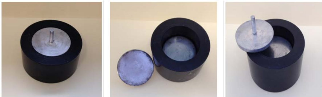
Figure 11. Capacitor jig setup
