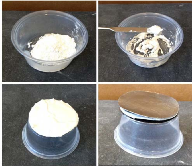
Figure 13. HSA capacitor assembly process
