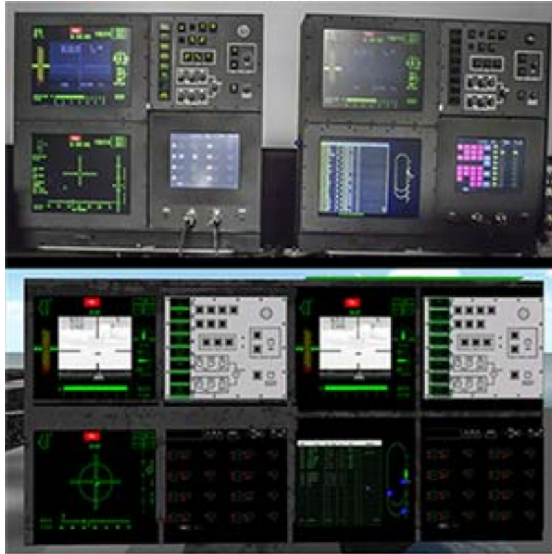
Figure 43. LSODS Comparison between 2H111 and LSO Prototype Trainer
