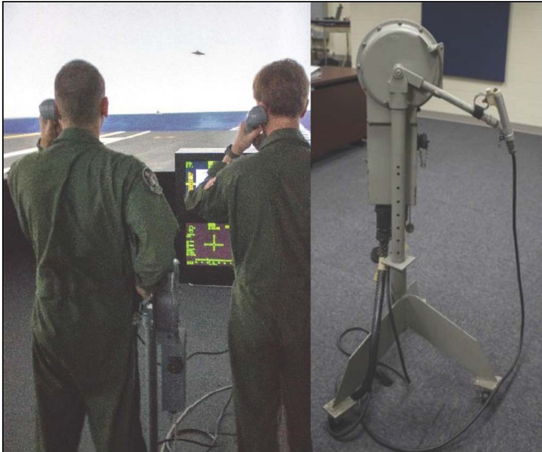
The Controlling LSO operating MOVLAS in 2H111 with Backup LSO Monitoring (left). MOVLAS rig with pickle attached (right).
