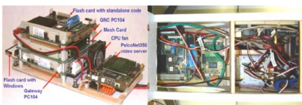
Fig. 10. Hardware integration and implementation architecture.
