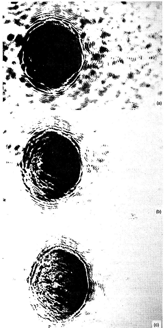
Fig. 4. Photographs of the near-field beam transmitted through the crystal at various times: (a) immediately after beam turn on, (b) during the process of beam fanning, and (c) just before the onset of self-pumped phase conjugation. Note that the scattering apparently begins at the periphery of the incident beam.
