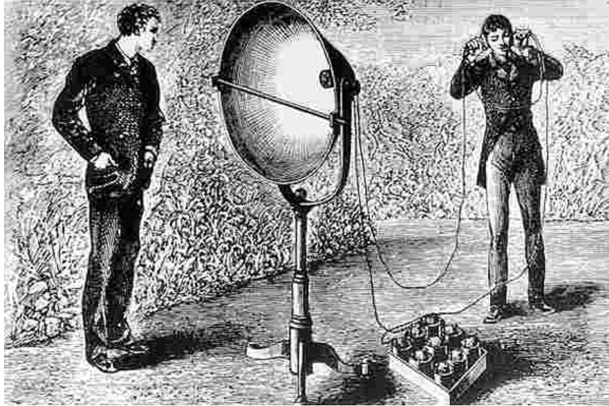
Figure 2. A photophone receiver, from [12].
