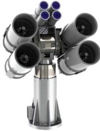
Figure 5. NASA LLCD ground terminal, from [17].
