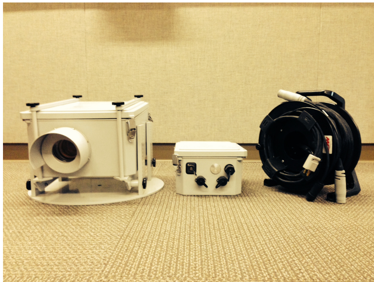
Figure 56. LaserFire V3 unit. Transmitter (left), modem (center), optical and power cable spool (right).
