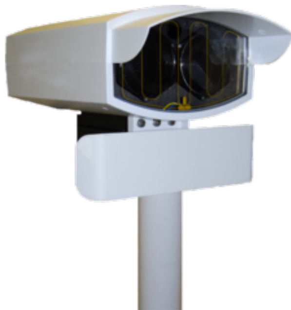
Figure 31. AireBridge SX with optional HyBridge radio, from [57].
