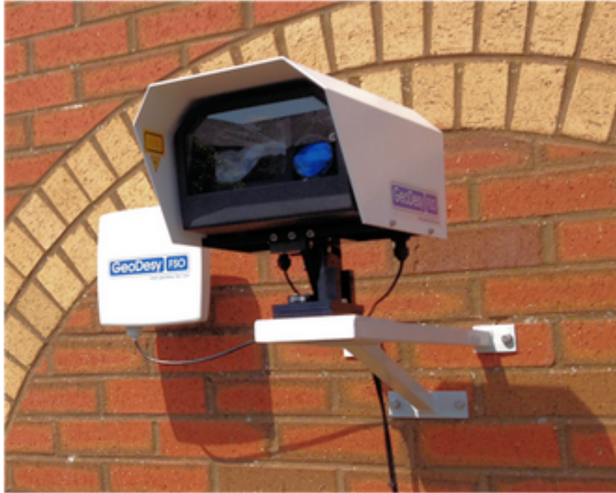
Figure 30. GeoDesy FSO system with optional RF backup, from [55].
