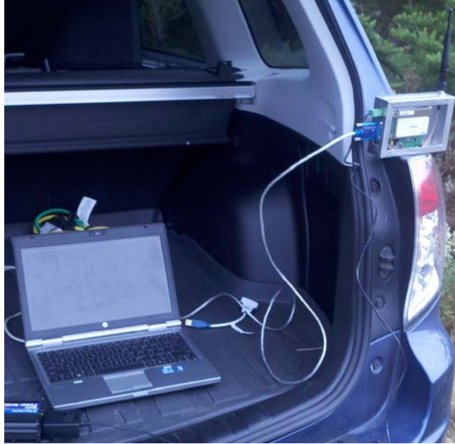
Figure 9. Mobile MHX-2400 radio system used for field testing
