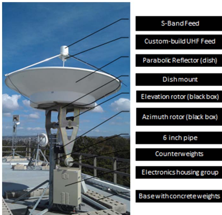
Figure 3. 3-meter dish system hardware
