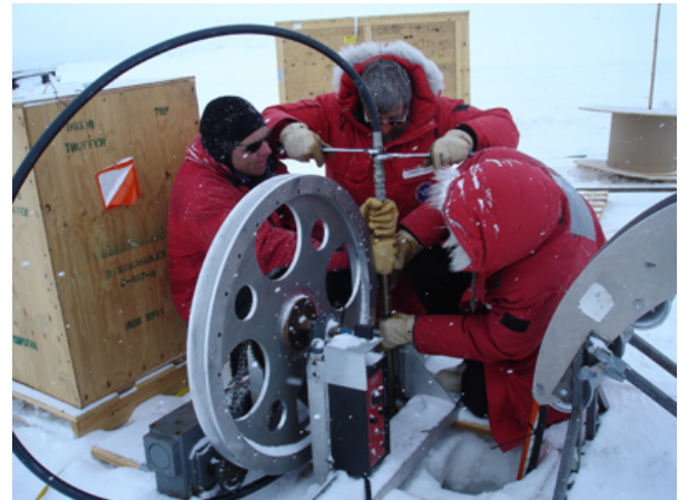
NPS Research Professor of Oceanography Tim Stanton, right, helps fellow researchers test the hot-water drill that will be used to create a tunnel for the ocean profiler. The researchers have made several trips to Antarctica to test the equipment in preparation for their current research trip, which will run from the end of Nov. through the end of Jan. (Photo provided by NASA)
